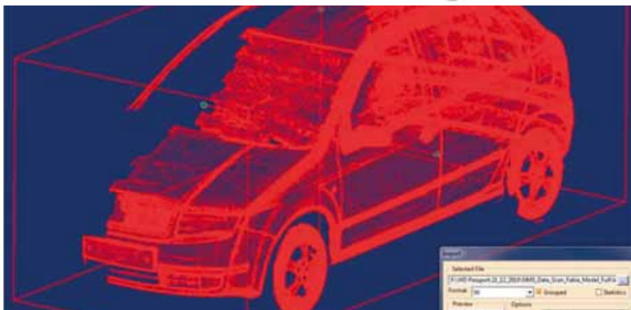
Obr. 9 - Importovanie mračna bodov v STL formáte do prostredia Digitized Shape Editor
