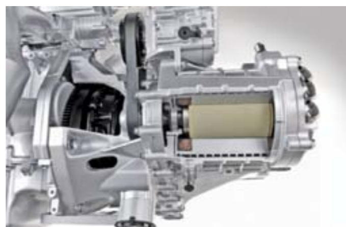
Obr. 11 Rez prevodovkou HDDCT s elektromotorom [8]
